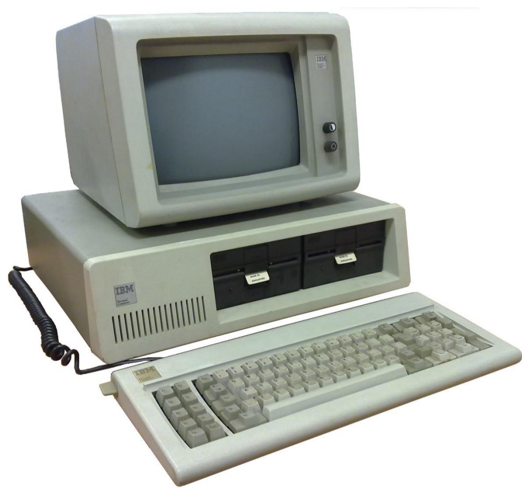
IBM PC model 5150: 1981-1987 CPU: Intel 8088 @ 4,77 MHz Memória: 16-256 kB
